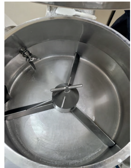
Figure 9: Cleaning success after the final washing cycle, phase 7.
