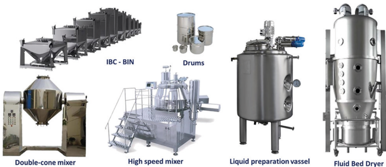
Figure 2: Examples of parts, bins, and vessels ready to apply high-pressure cleaning as CIP method.
