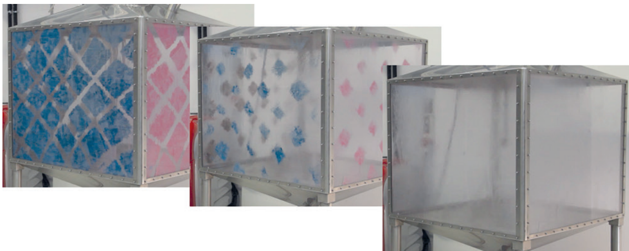
Figure 5: Cleaning exposure pattern of hydrokinetic lance with 4 nozzles.
