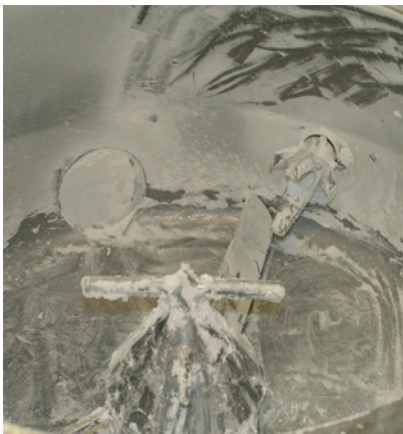
Figure 8: Initial contamination of the Rapid Mixer Granulator and its interior tools.
